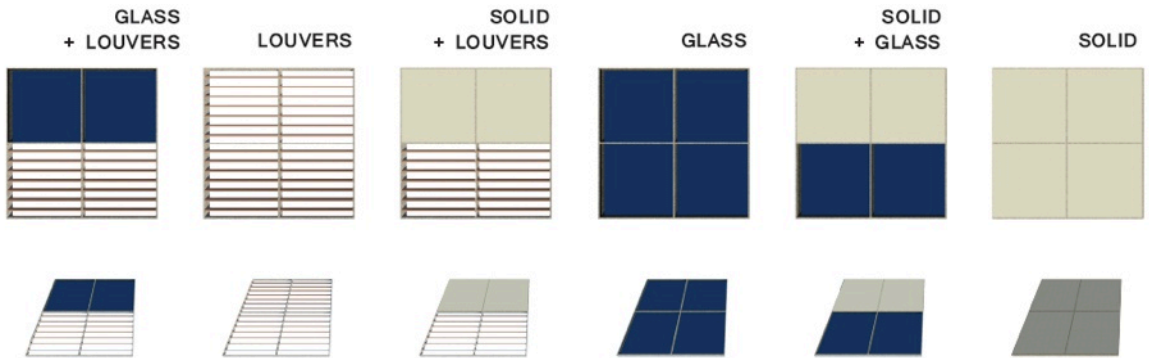
Figure 41: Roof Panel Types
